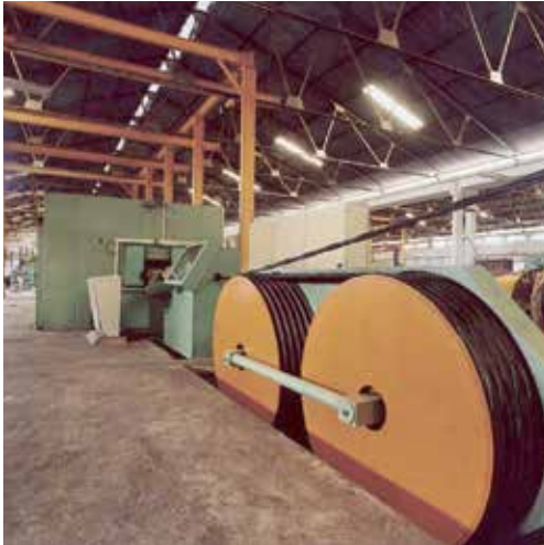
Assembly of an Aerial Bundled Cable on a Bow strander machine at 180m/min
