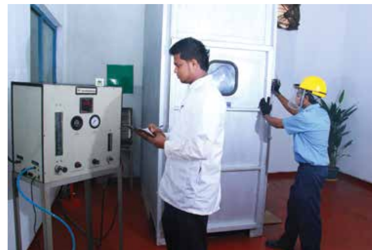
Testing of vertical flame spread of vertically mounted bunched wires or cables .
