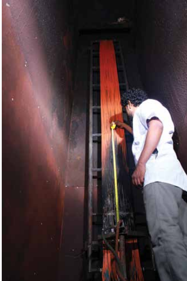
Measuring of the vertical flame propagation of low smoke halogen free power cables.
