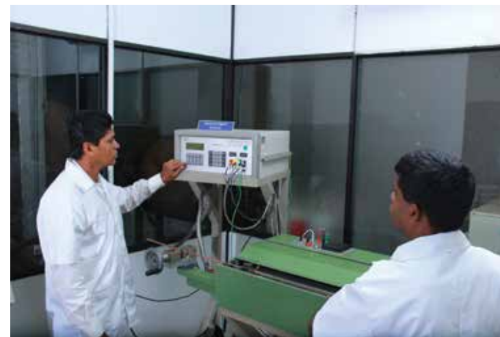
High precision automatic Resisrana Bridge used for the measurement of electrical resistance of Power - X Cables up to 1000 mm 2
