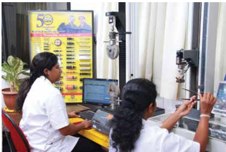
Electronic Tensile Tester - To Obtain tensile strength & elongation values of Power - X Cables up to 4 x 400 mm 2 .
