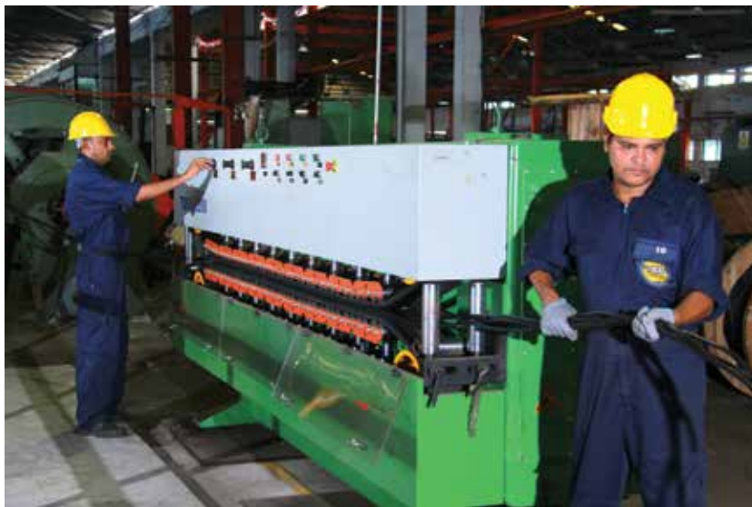
Heavy duty, high boddin weight, Planetary Strander line for assemblins of LA / MV Aerial Bundled Cables
