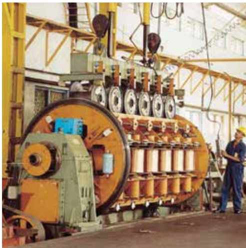
Batch loading of Copper wires in 630 DIN Spools on 61 strand high speed Tandem Strander.
