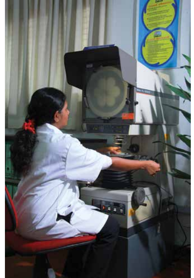
Profile Projector & Digimatic mini Processor - To obtain accurate measurement of thickness of insulated cores of Power - X Cables.
