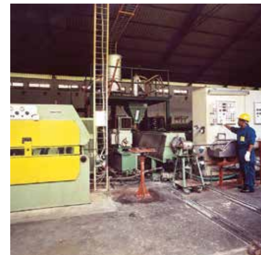
Extrusion of outer sheath of 4x400mm 2 at the rate of 800kg of PVC per hour on an 120mm Extruder.
