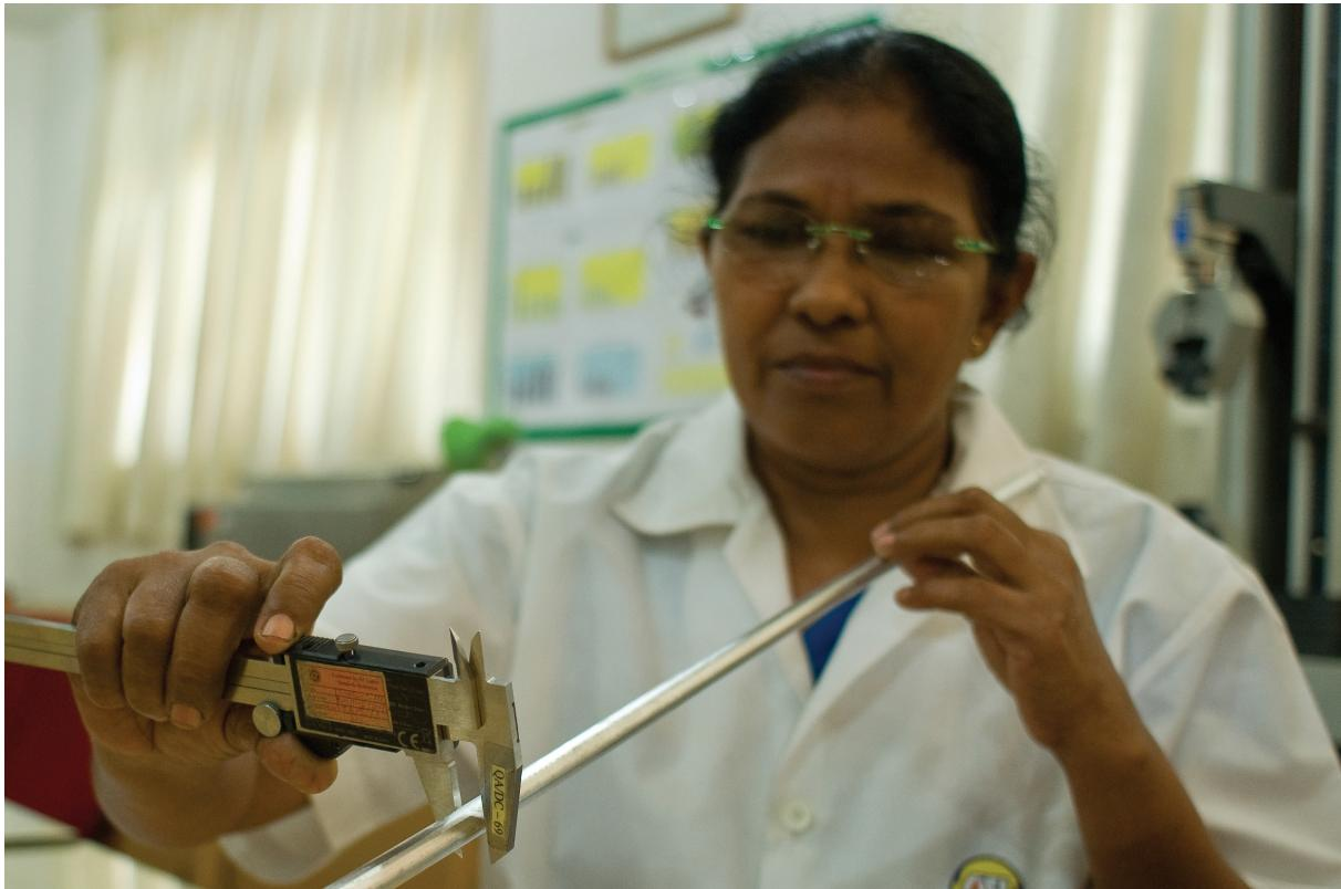
*Measuring of Physical Parameters of Finished Aluminium Rod*
