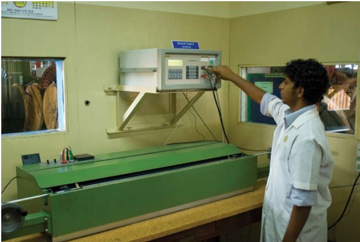
Automatic Temperature Controlled Equipment for measurement of Resistance of conductors
