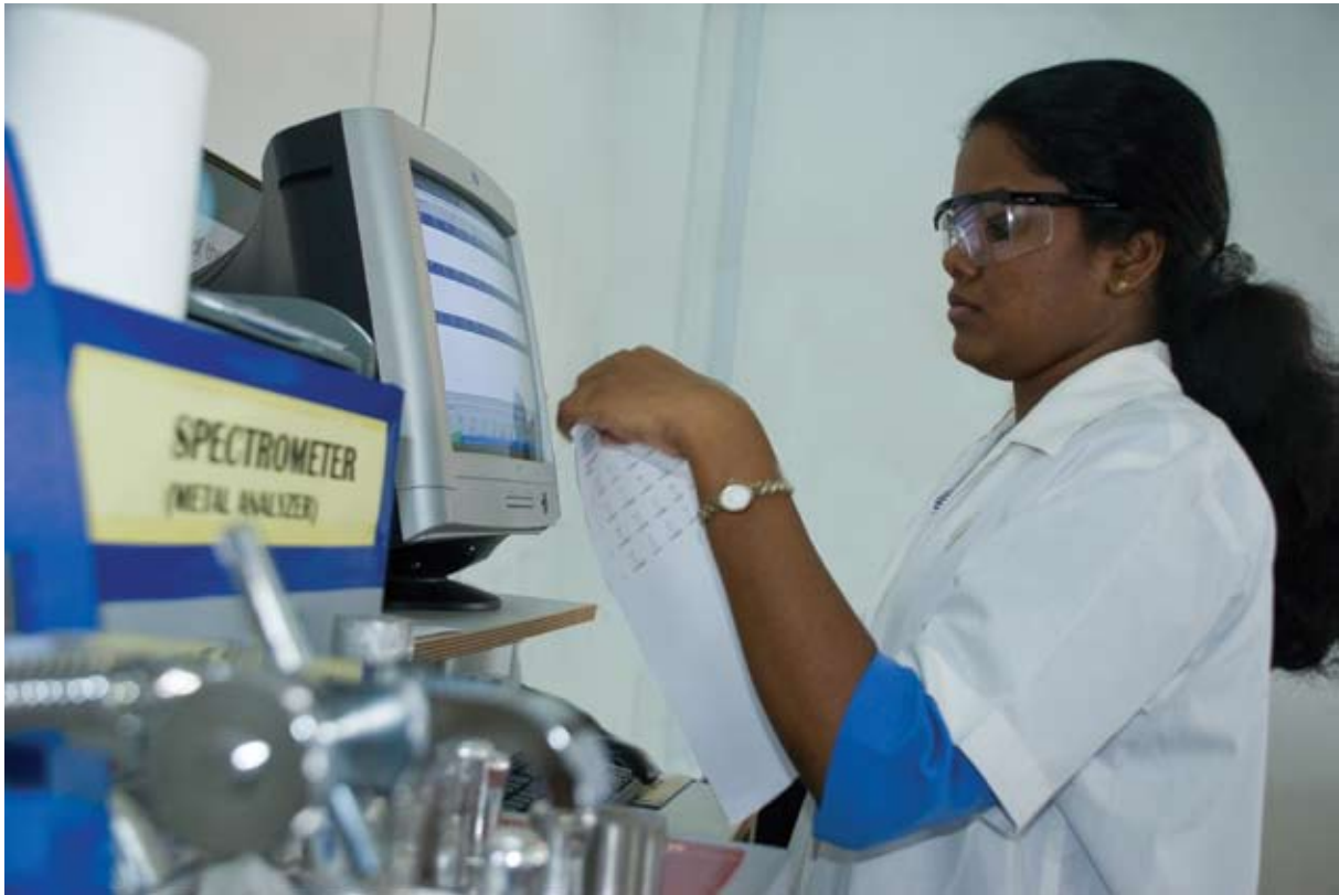
Optical Emission Spectrometer for analyzing chemical composition of Aluminium
