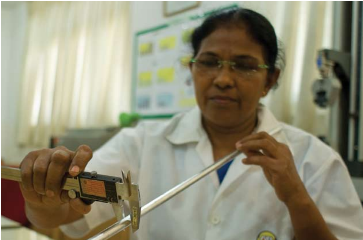
Measuring Physical Parameters of Finished Aluminium Rod
