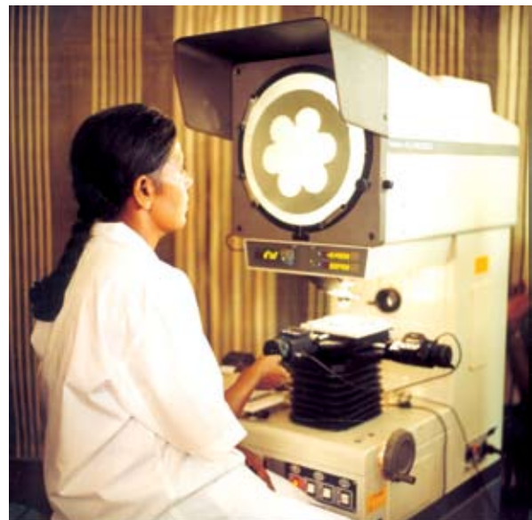
Profile Projector being used to measure insulation thickness of ABC
