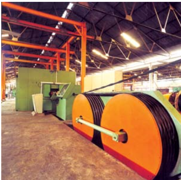
Aerial Bundled Cable is being assembled on Bow Cabler
