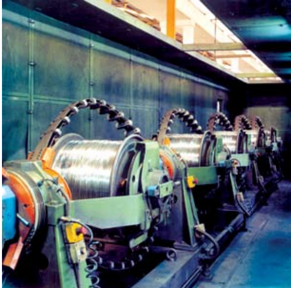
7 Strand Aluminium Conductor is being stranded on Skip strander
