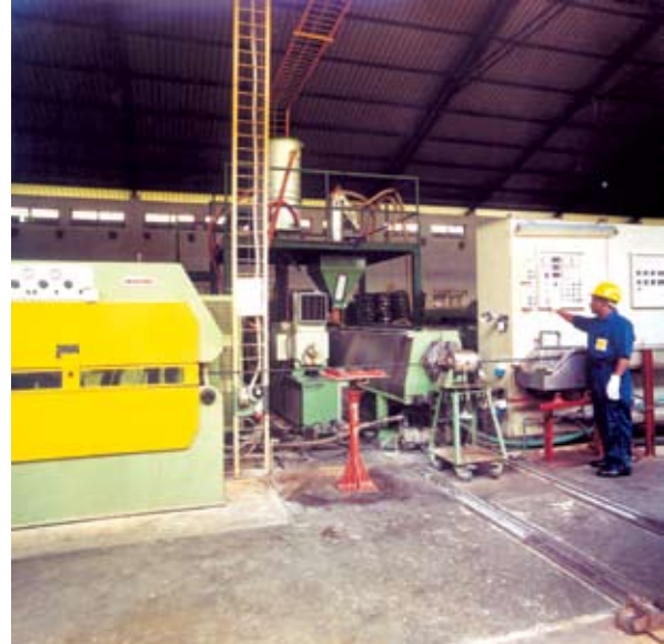
A phase conductor is being extruded with XLPE
