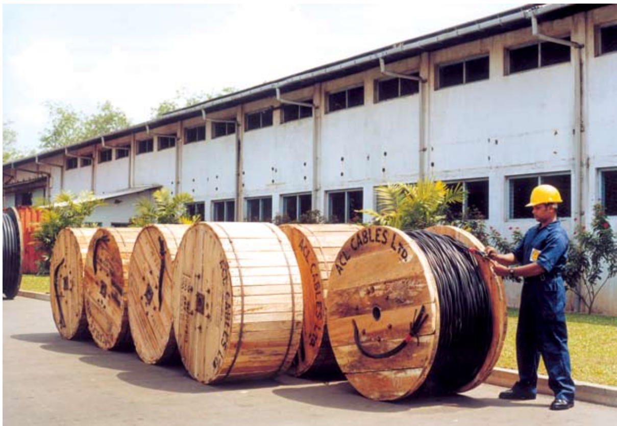
Aerial Bundled cables packed in drums at ACL yard being inspected before despatch
